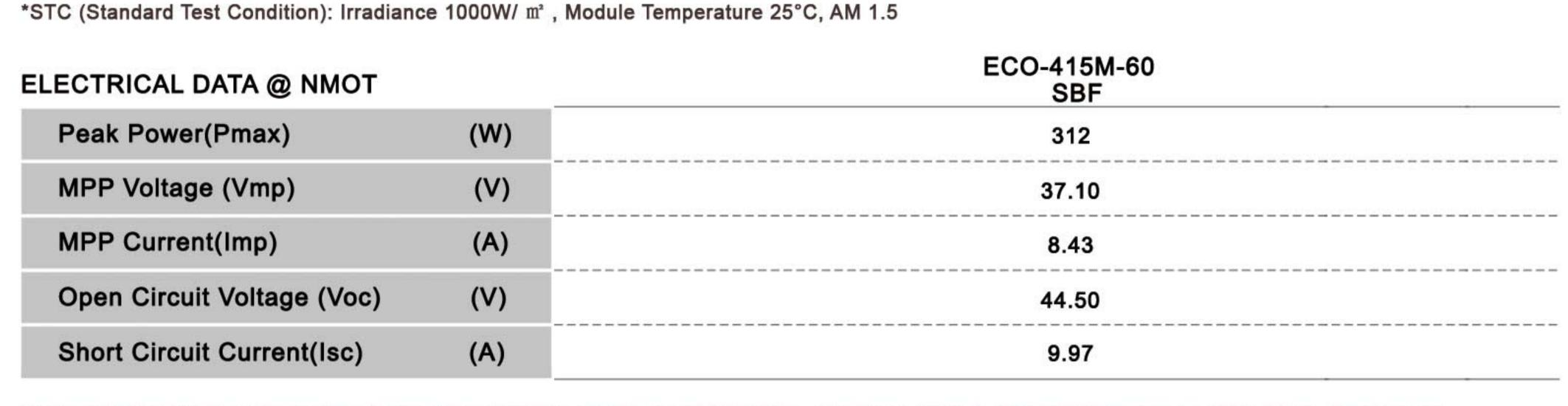
\*Under Nominal Module Operating Temperature (NMOT), Irradiance of 800W/ m², Spectrum AM 1.5, Ambient Temperature 20°C, Wind Speed 1m/s
