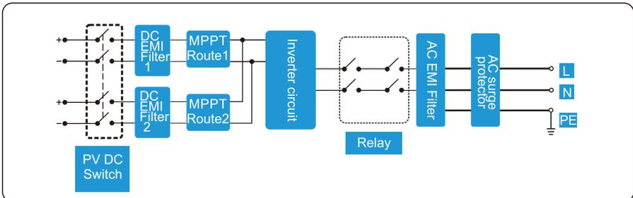
Figure 2.9 circuit diagram
