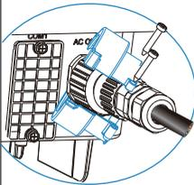
After the **type B** terminal is connected, install protection sleeve on the connection position, and tighten the screws to prevent the terminals from slipping off.
