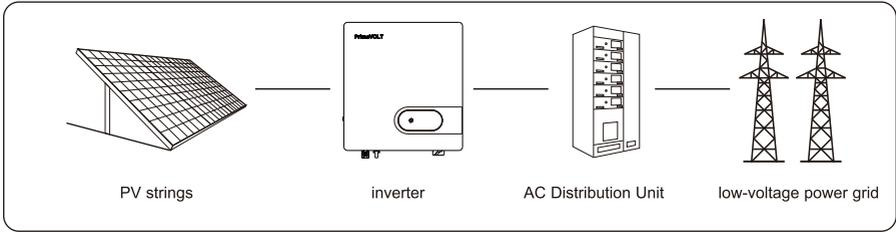
Figure 2.2 A low-voltage grid-tied PV power system
